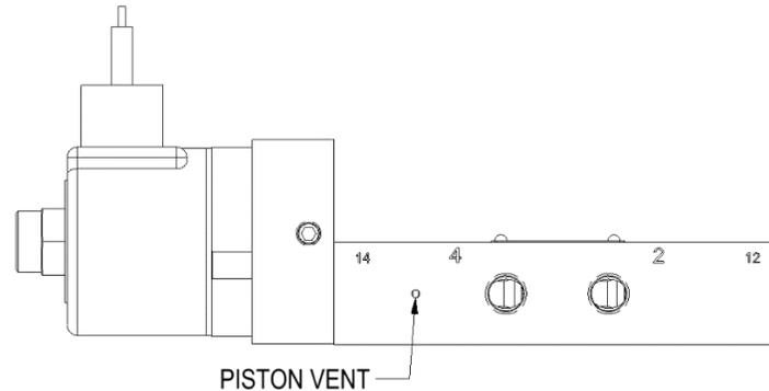
Vent leakage when the solenoid is energized can be caused by either a faulty operator piston or cap seal. Contact the factory.
