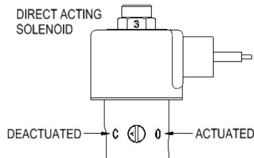
If a turn locking manual override is left in the actuated position, the valve will operate when the override is again cycled, from on to off and back to on, but will fail to operate electrically. This happens because the override is holding the plunger in its actuated position.
