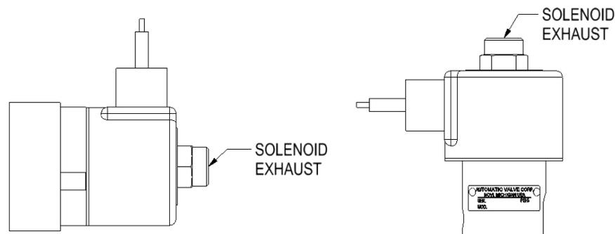
Continuous leakage from the operator exhaust port when the solenoid is de-energized can be caused by a foreign particle trapped between the bottom seat and the plunger, by a damaged bottom seat, or by a worn or damaged bottom plunger seal.
