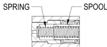
Broken springs on spring return valves can cause a valve to remain in the actuated position or to only partially return and perhaps leak to exhaust.
