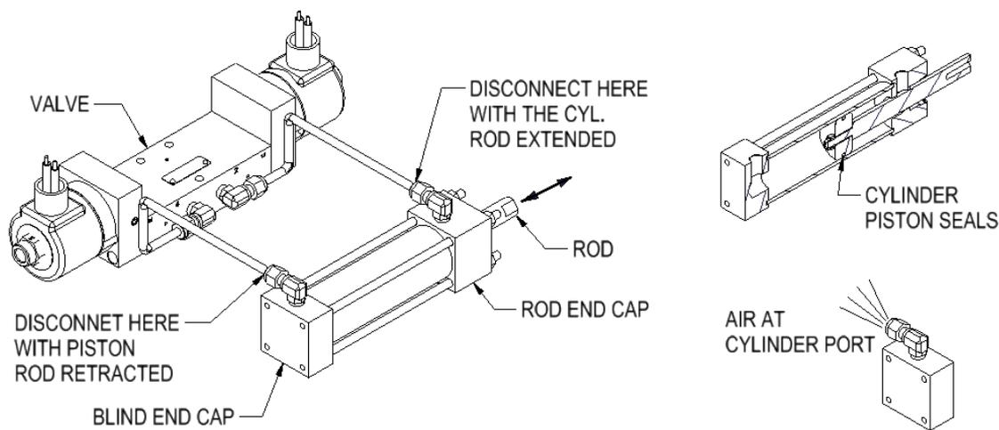
Verify if the leakage is caused by the cylinder or valve as follows: (Use extreme caution as the valve and cylinder will both be actuated during this procedure.)
